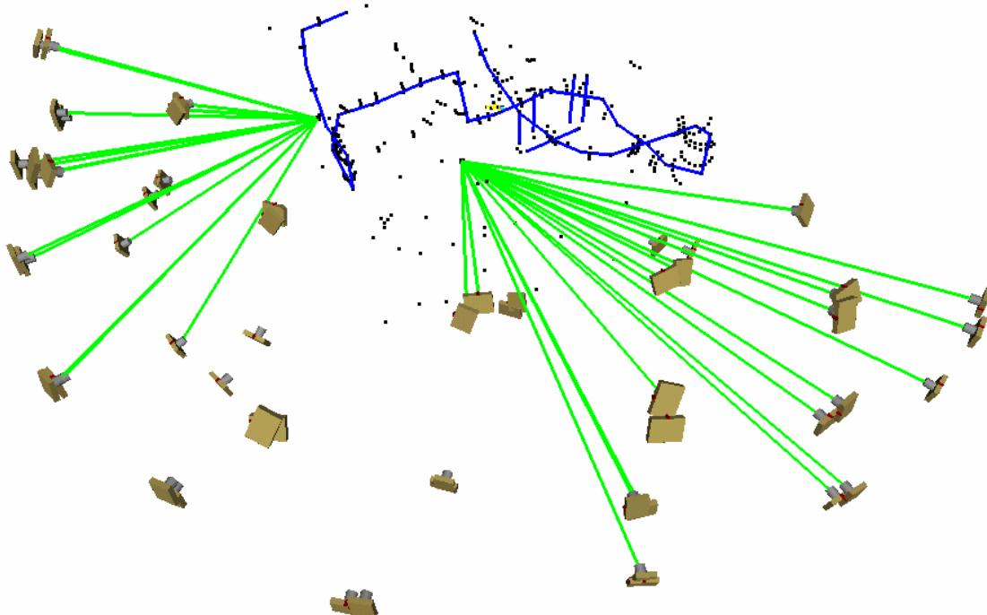
Approximately 55 photographs were taken of the work volume. With planning this number can be reduced to approximately 40 depending on the complexity of the measurement and accuracy requirements.
