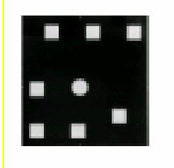
To automate the measurement process it was necessary to add "coded" targets to the pipes and surrounding volume. These targets are automatically detected and help the software determine the location and orientation
