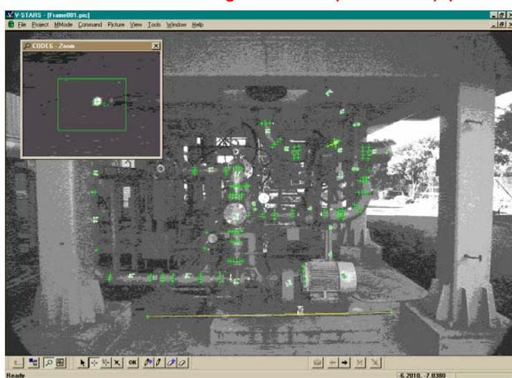
The green text represents points that have been located in this particular image. Note that the image appears very dark and difficult to see. This is intentional as the best photogrammetric measurements are made on images that have dark backgrounds and bright targets. One of these targets is shown in the zoom window in the top left-hand corner.
