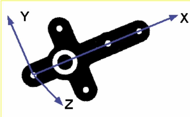
the bottom of the AutoBar. The positive Y-axis goes through Target 3 at the top of the bar. The positive Z-axis is up out of the AutoBar. The diagram on the left shows both the AutoBar and its coordinate system
