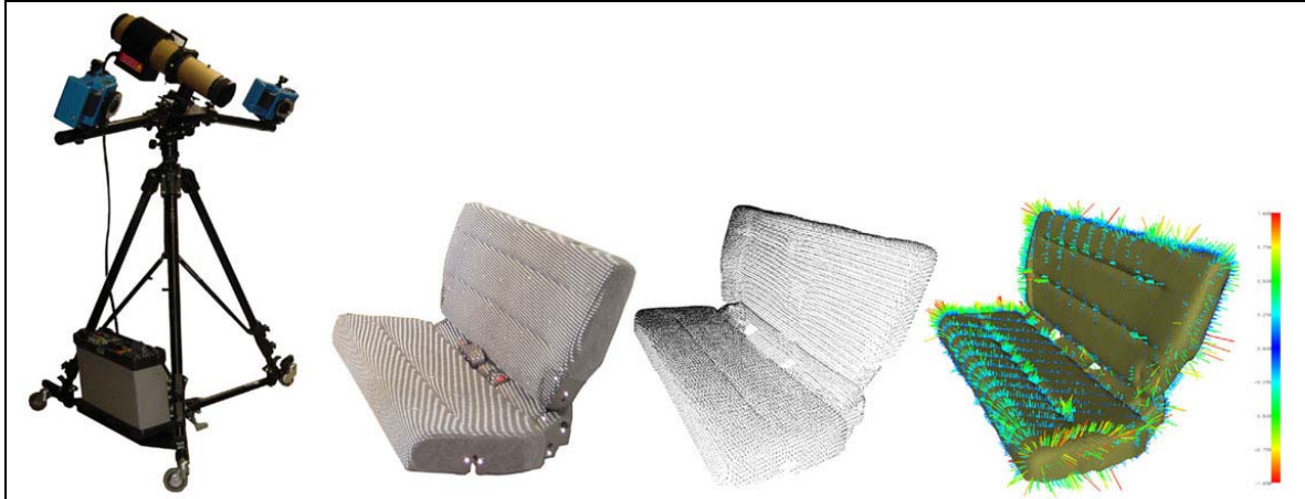
V-STARS being used to measure and verify a car seat.
