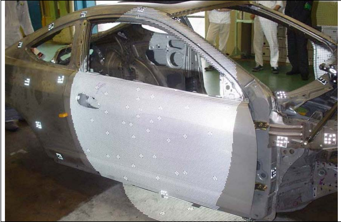
Typical surface measurement to verify door position
