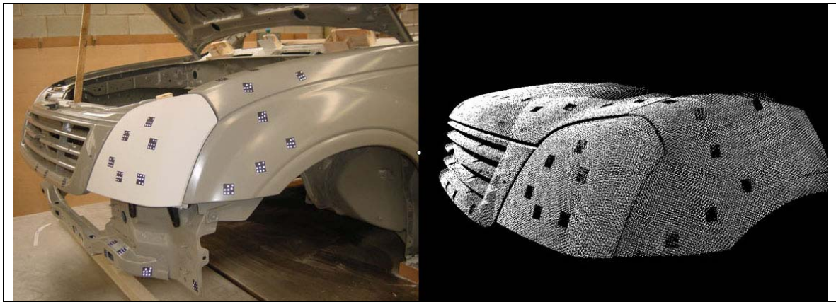
PRO-SPOT being used to measure the location of a head light and grill relative to the car body.
