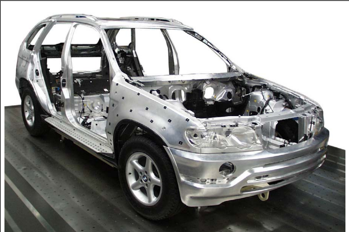
BMW X5 master model used as a test bed for individual parts
