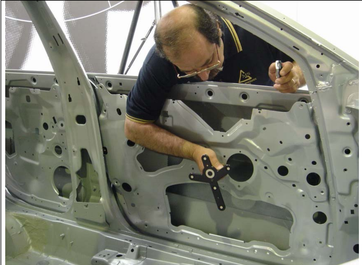
Operator using hand-held probes to determine key hole location on Audi door
