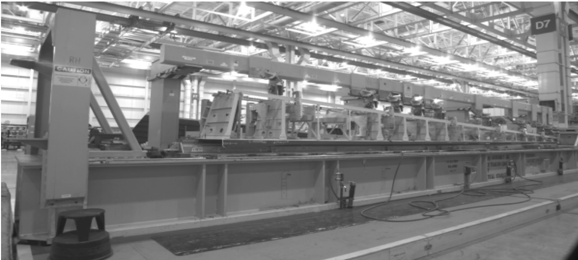
Figure 4a – Empennage Assembly Tool used for acceptance test
