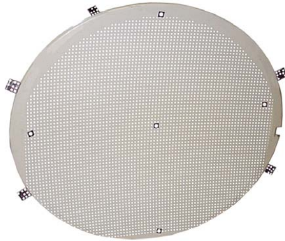
FIGURE 8 – Antenna showing projected targets.
